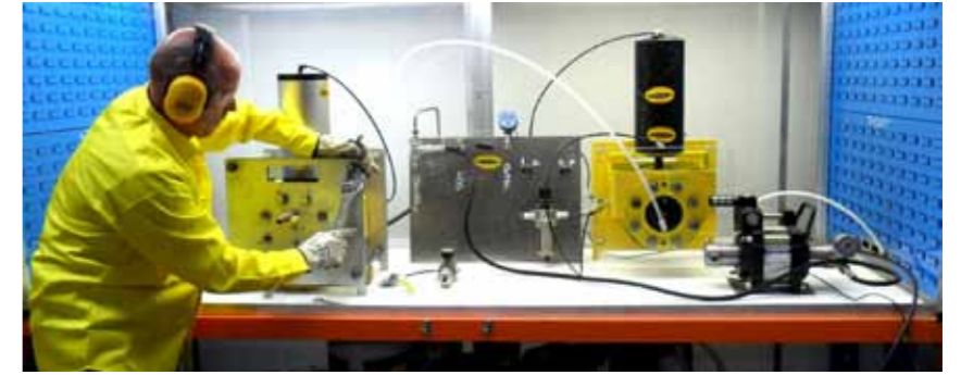
Pressure testing sleeves under controlled conditions
