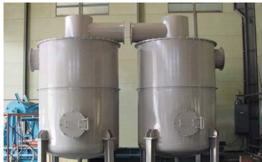
1st Mist & Dust Collector
