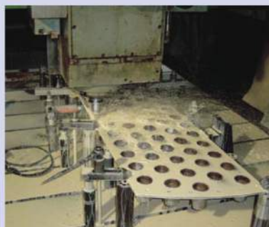
FINAL BOLT HOLE DRILLING FOR DISTRIBUTOR TRAY
