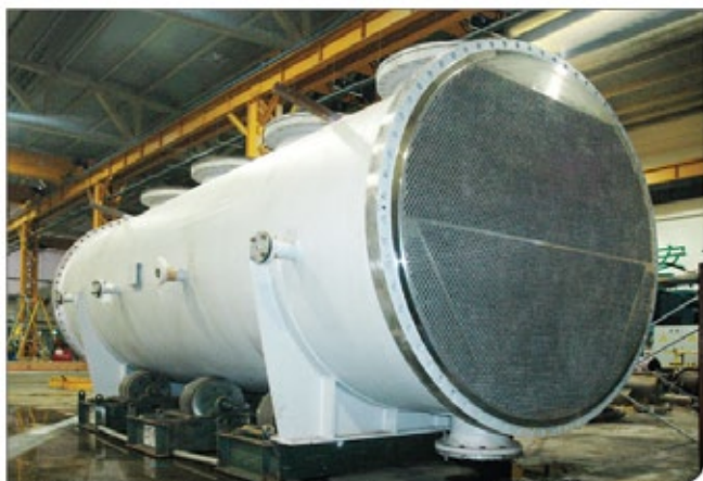
This 55 tons stainless steel heat exchangers with 7775 tubes, shell dia 2200mm complete shell side hydrotest.
