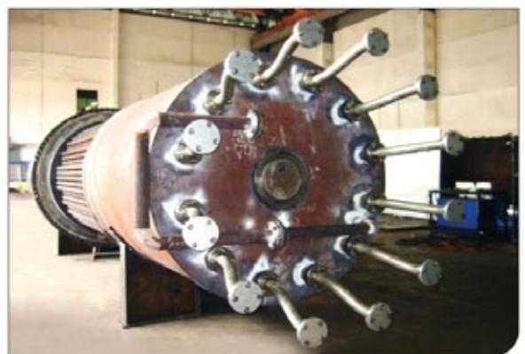
This 23 tonnes CCR Reduction Zone Exchangers is constructed with combination of CrMo P5, P22 and SS321 material.
