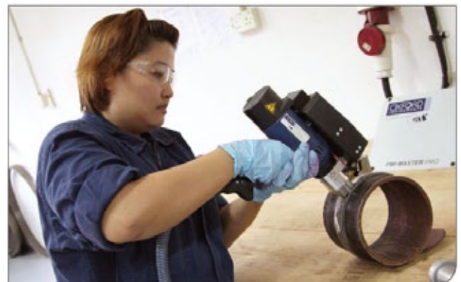
PMI-Master Pro (Able to detect carbon content)
