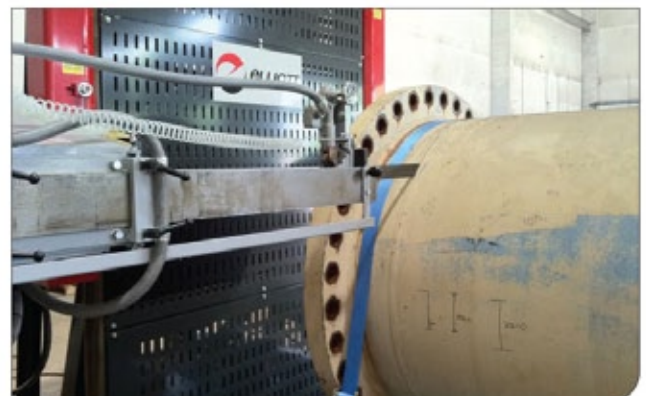
Bandsaw machine for quick & clean cut up to maximum OD 2,500mm.
