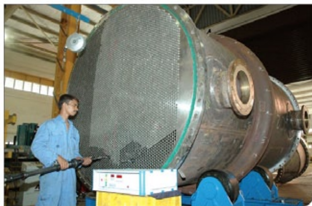
Digital Torque control expansion assure equal torque being apply to each tube, thus prevent over or under expansion & improve productivity.
