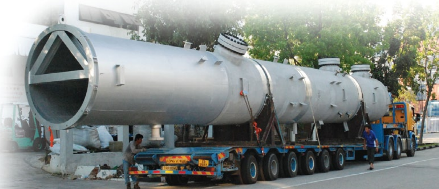
Clad 316L column with diameter 2m x length 22m x weight 60 tons.
