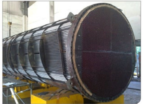
This Alloy 200 (99% nickel) U-bundle is constructed with double tube sheet.
