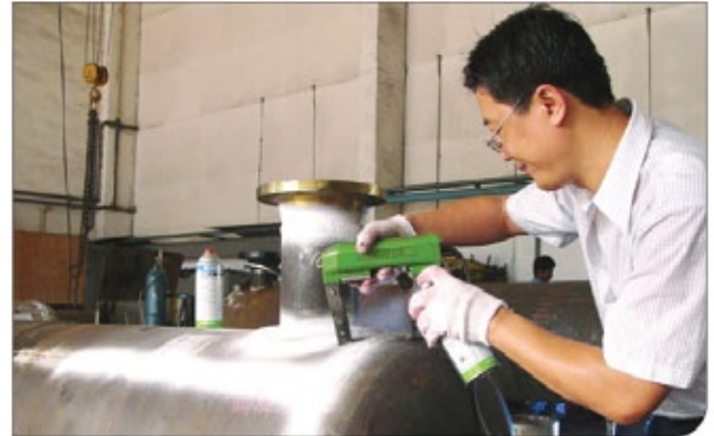
Magnetic Particle Test is able to pick up hair line cracking.
