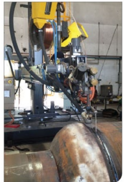
Submerge Arc Welding for heavy wall vessel.
