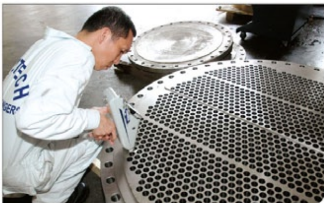
PMI testing ensure right composition of base material & welding consumable being use.
