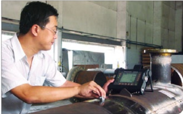
Our in-house Level III QA is performing UT test on a shell body.
