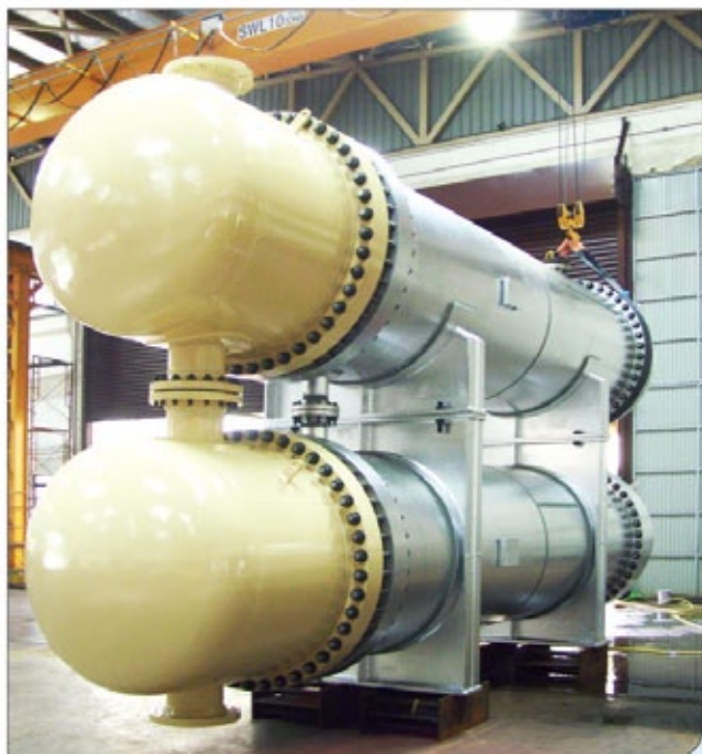
Hydrotest of stacked type heat exchangers as per API 660.
