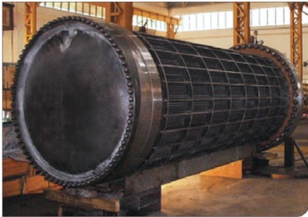
A removable duplex stainless steel tube bundle with floating head (AES Type).
