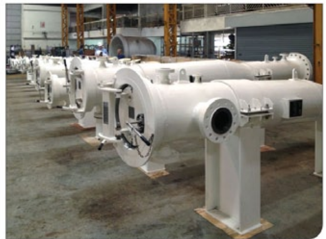
PIG Launchers & Receivers with Quick Opening Closures (QOC) are fabricated for the cleaning of pipelines internal wall surfaces.
