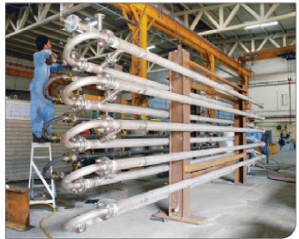
These double pipe hairpin exchangers are constructed with fin material welded on longitudinal axis by High Frequency Welding.
