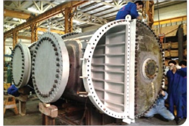
Pressure vessel with special GRP lining for the internal coating.
