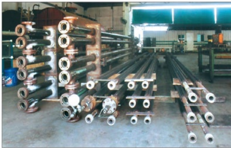
These double pipe hairpin exchangers are constructed with fin material welded on longitudinal axis by High Frequency Welding.
