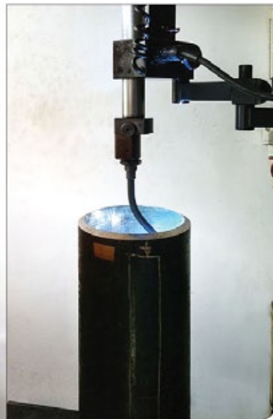
FCAW, DSS filler for inside pipe weld overlay.
