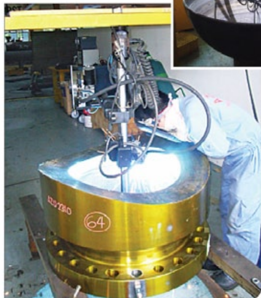
The new overlay welding machine able to deposit alloy over carbon steel tubesheet & pipe.
