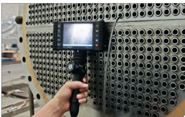
Vedioscope to check tube internal to enhance product quality.
