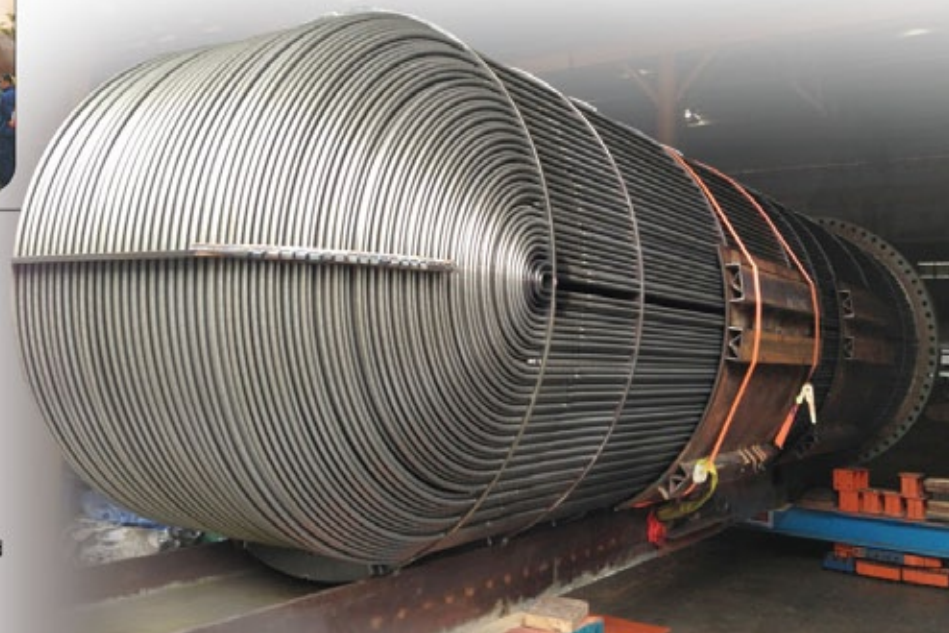
SA179 U-tube bundle with Special Internal & External tube finings (3044 pcs) to be inserted into Shell using bundle puller.
