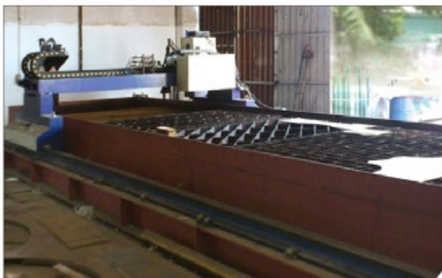
CNC profile cutting machine for plate cutting.
