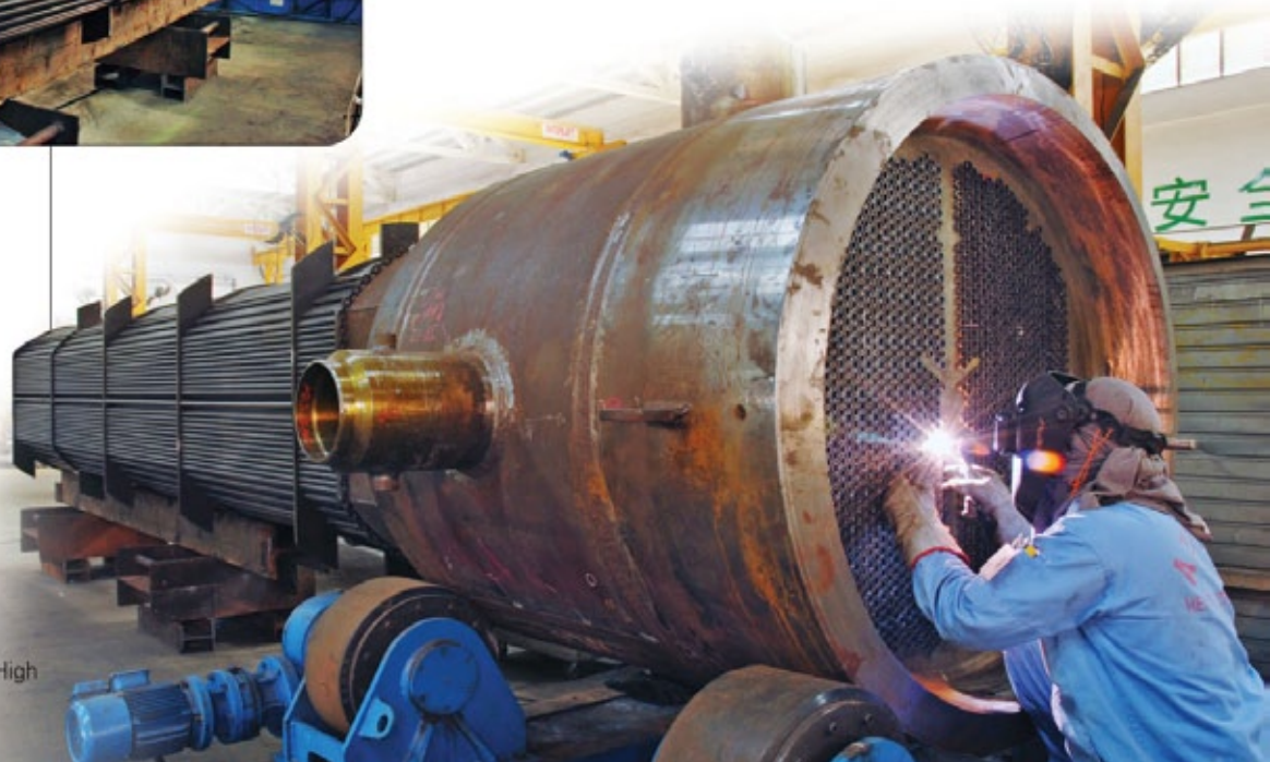
A special design Flanged-only Tubesheet U-bundle sits on a rotator for final dimension inspection. Tube side hydrostatic test pressure up to 167 barg.
