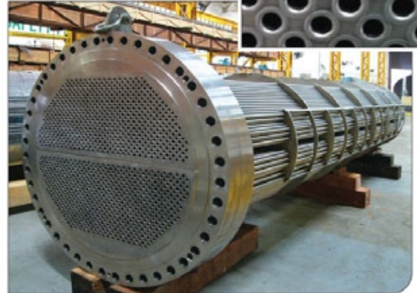
A Completed titanium U-bundle with tube to tubesheet welding.
