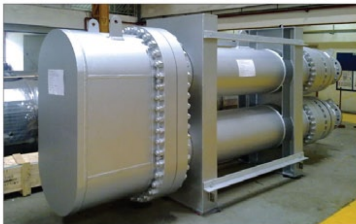
A multi-tube high pressure return cover by plate forming & welding.
