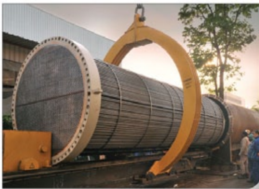
Retubing of SA179 Helical U-tube bundle (2553 pcs) within 2 weeks with tube end strength welding.
