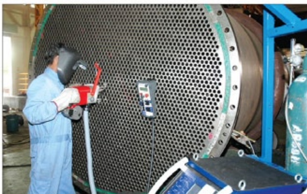
New auto welding machine able to weld Titanium tube.
