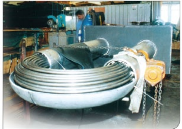
Complete Hastalloy C276 Multi-tube Hairpin economizer for CO 2 to CO 2 application (U stamp).
