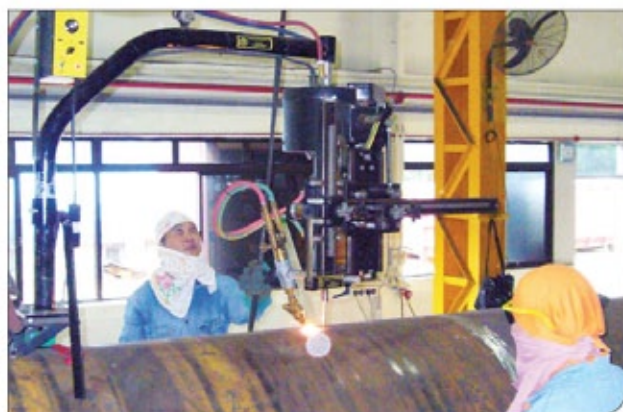
Profile cutting machine for thick wall shell nozzle opening.
