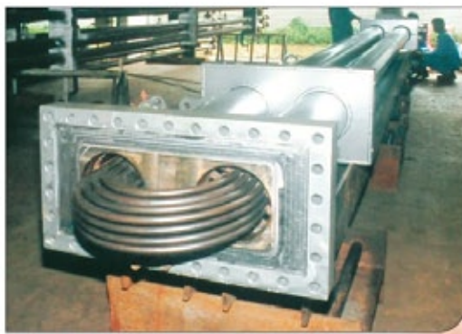
These double pipe hairpin exchangers are constructed with fin material welded on longitudinal axis by High Frequency Welding.
