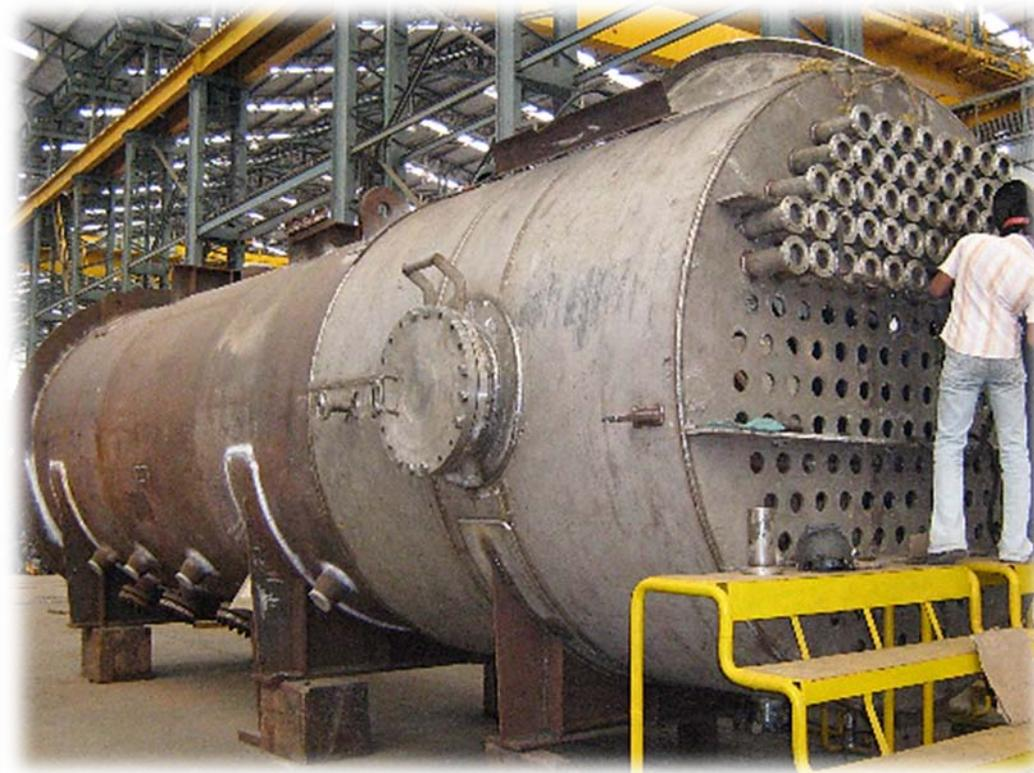
Waste Heat Boiler Lance Ports for Tube Cleaning
