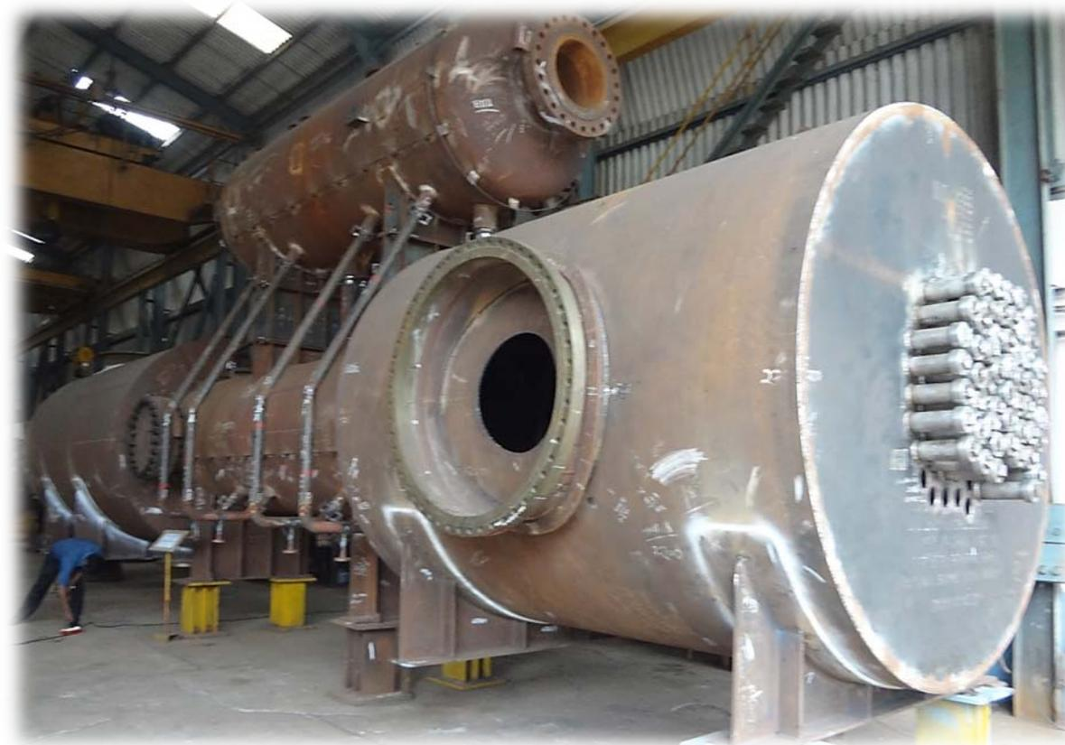
Waste Heat Boiler with Steam Drum under Trail Assembly at workshop
