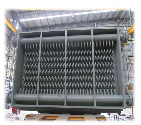
Superheater Module under fabrication
