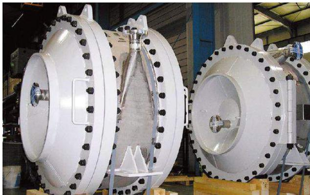
PVC Slurry Heat Exchanger
