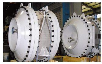
PVC Slurry Heat Exchanger
